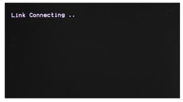
h)The system will spend 20-30 seconds on constructing the link, and real link period will depend on the current wireless channel condition. When wireless link is set up, "RSSI" light will light and indicate current received wireless signal strength, as well "Video" indicators will light, and then connected HD monitor will display the video and audio accordingly.
