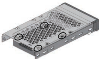
Figure 1-4-1. Installing 2.5-inch SAS/SATA Drive
