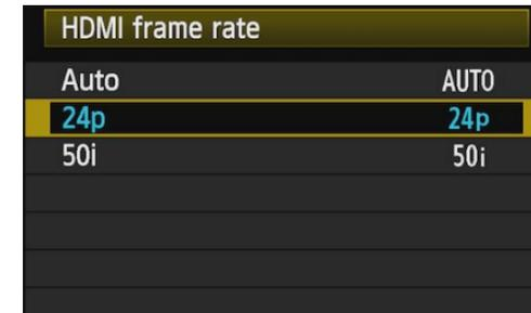
*Note: The required HDMI format is related to (clean) HDMI output, not the Record format.*
