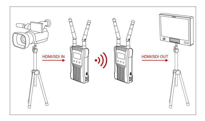
This wireless HD video transmission system uses the latest wireless communication technology and transmits ultra-low latency HD video. The transmitter supports both HDMI and SDI input, while the receiver supports both HDMI and SDI output. It is configurated with OLED display screen and supports iOS & Android App Monitoring.
