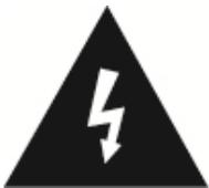
This symbol indicates the presence of un-insulated, dangerous voltage inside the enclosure of the charger. There is a risk of shock if the charger case is opened.
